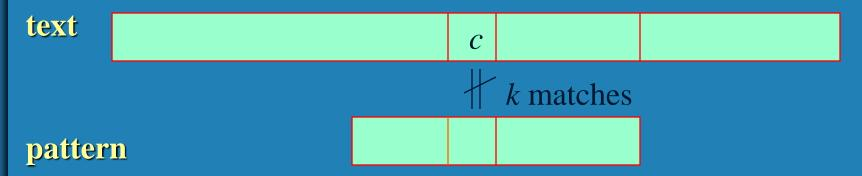
■ bad-symbol shift  $d_1 = \max\{t_1(c) - k, 1\}$ , where  $t_1(c)$  is precomputed by Horspool's algorithm
