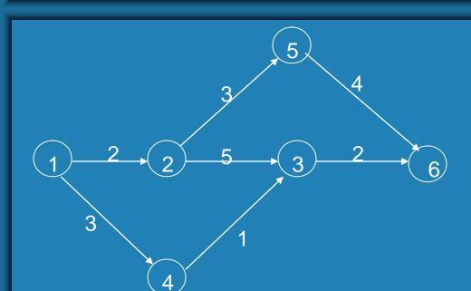
If X = {1} and  $\overline{X}$  = {2,3,4,5,6}, C(X, \overline{X}) = {(1,2), (1,4)}, c = 5 If X ={1,2,3,4,5} and  $\overline{X}$  = {6}, C(X, \overline{X}) = {(3,6), (5,6)}, c = 6 If X = {1,2,4} and  $\overline{X}$  ={3,5,6}, C(X, \overline{X}) = {(2,3), (2,5), (4,3)}, c = 9
