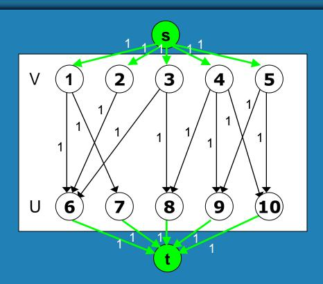
Add a source and a sink, direct edges (with unit capacity) from the source to the vertices of V and from the vertices of U to the sink
