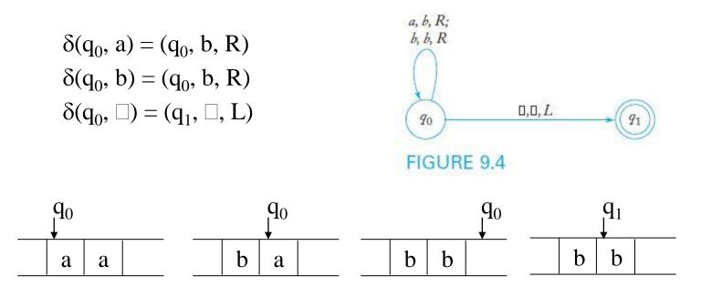
A sequence of moves as the machine processes a tape with initial contents aa
