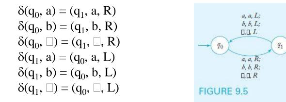
This machine with input string ab runs forever —in an infinite loopwith the read-write head moving alternately right and left, but making no modifications to the tape
