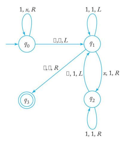
Example 9.11: Let x and y be two positive integers represented in unary notation. Construct a Turing machine that will halt in a final state  $q_y$  if  $x \ge y$ , and that will halt in a non-final state  $q_n$  if x < y.
