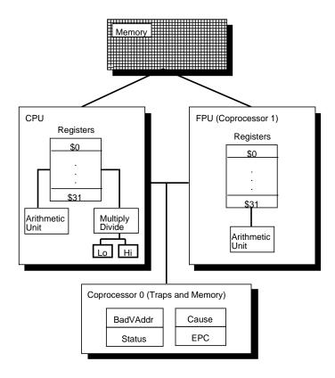
Figure 2: MIPS R2000 CPU and FPU
