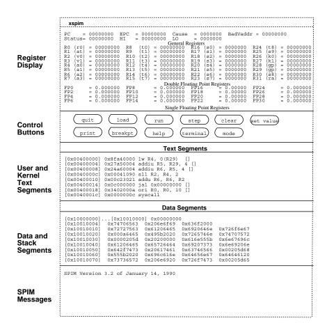
Figure 1: X-window interface to SPIM.
