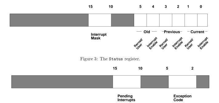
Figure 4: The Cause register.
