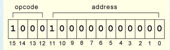
• We see that the opcode is 8 and bits 11 and 10 are 10, meaning that the next instruction will be skipped if the value in the AC is greater than zero.
