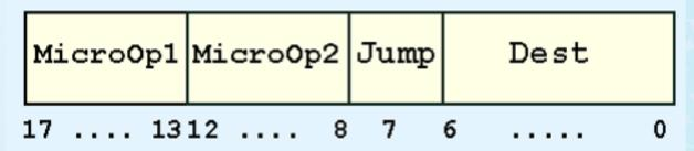
MicroOp1 and MicroOp2 contain binary codes for each instruction. Jump is a single bit indicating that the value in the Dest field is a valid address and should be placed in the microsequencer.
