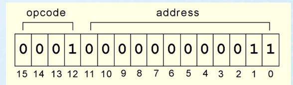
• We see that the opcode is 1 and the address from which to load the data is 3.
