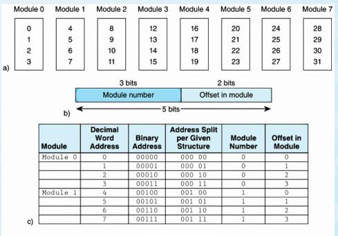
a) High-Order Memory Interleaving b) Address Structure c) First Two Modules
