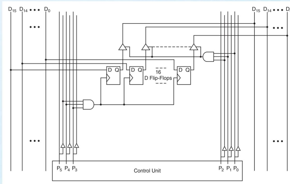
The register MBR is enabled for reading when  $P_0$  and  $P_1$  are high, and enabled for writing when  $P_3$  and  $P_4$  are high.
