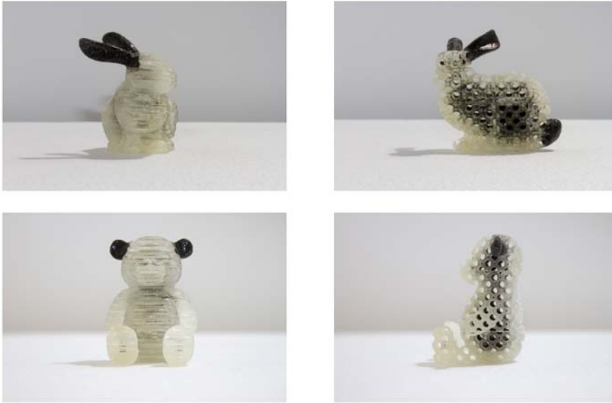
Images from: Openfab: A programmable pipeline for multi-material fabrication (Vidimče, K. et al. 2013) demonstrating a repeating hollowing pattern copied from one model and reused on another model.
