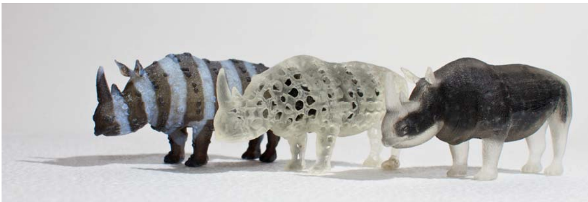
Images from: Openfab: A programmable pipeline for multi-material fabrication (Vidimče, K. et al. 2013) demonstrating how different fablets can be loaded onto the same model to create different, repeatable results.
