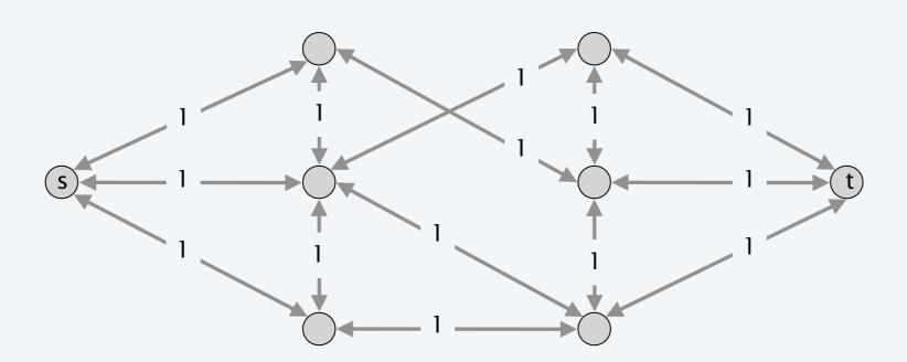
Max flow formulation. Replace edge edge with two antiparallel edges and assign unit capacity to every edge.
