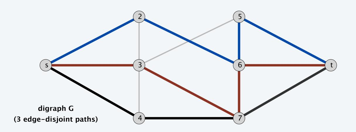
Max flow formulation. Replace edge edge with two antiparallel edges and assign unit capacity to every edge.
