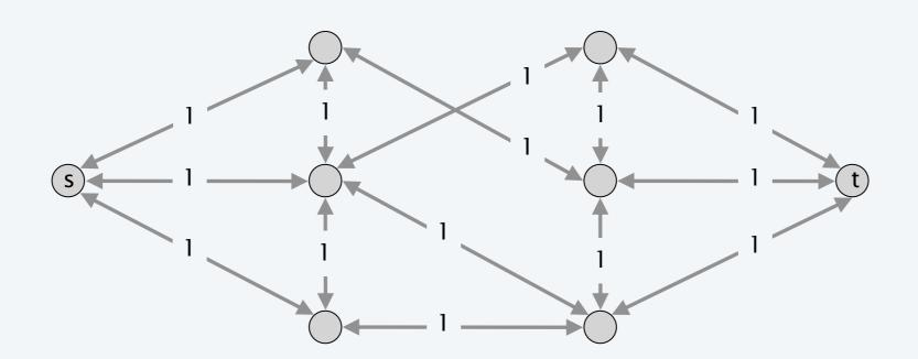
Max flow formulation. Replace edge edge with two antiparallel edges and assign unit capacity to every edge.
