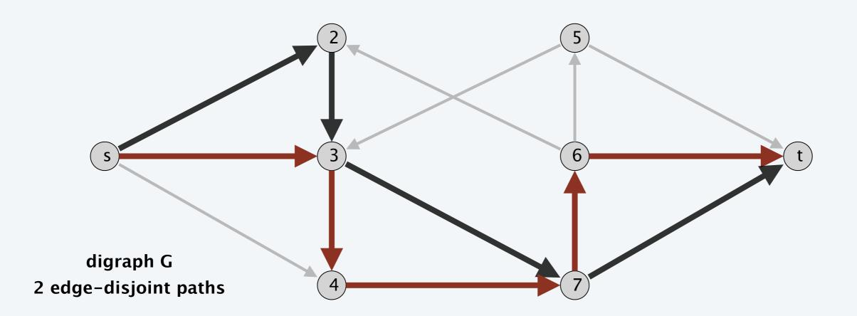
Max flow formulation. Assign unit capacity to every edge.
