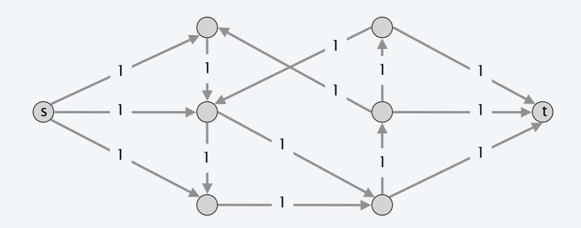
Max flow formulation. Assign unit capacity to every edge.
