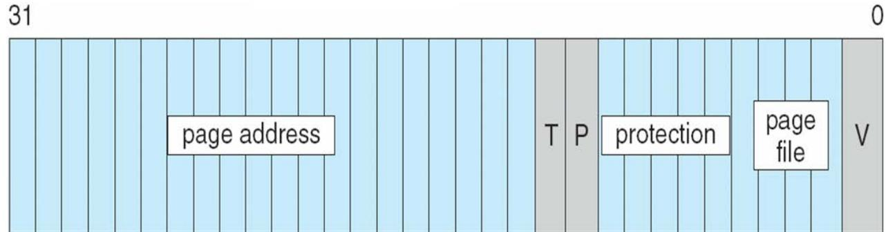
5 bits for page protection, 20 bits for page frame address, 4 bits to select a paging file, and 3 bits that describe the page state.  $V = 0$
