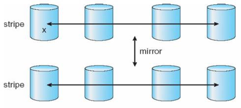
a) RAID 0 + 1 with a single disk failure.
