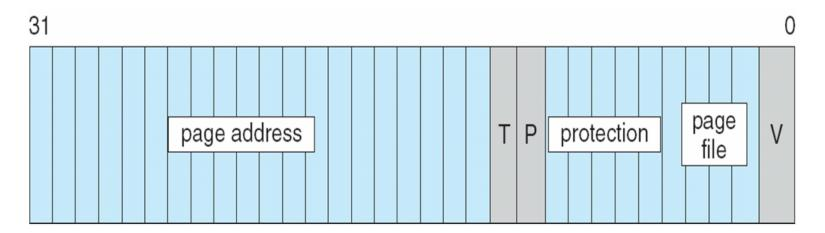
5 bits for page protection, 20 bits for page frame address, 4 bits to select a paging file, and 3 bits that describe the page state
