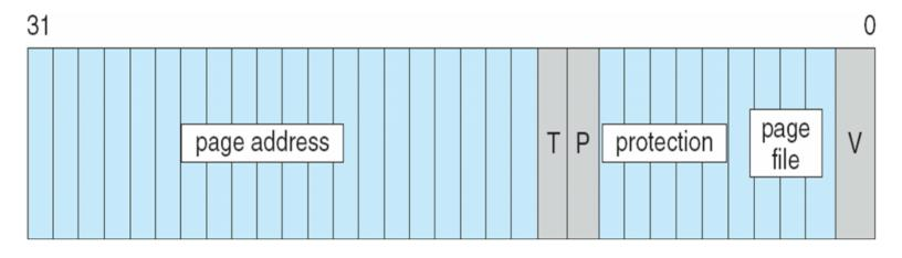
5 bits for page protection, 20 bits for page frame address, 4 bits to select a paging file, and 3 bits that describe the page state. V = 0
