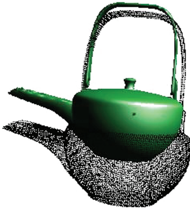
Figure 16: Point data set used for reverse construction (black) and an intermediate shape during the fitting process (green).
