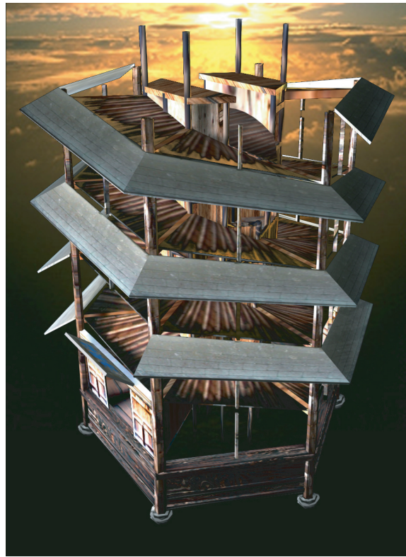
Figure 5: Exterior tower's double-helical exterior overhangs and interior walkway with exterior walls removed; textured model by B. Britton [7].
