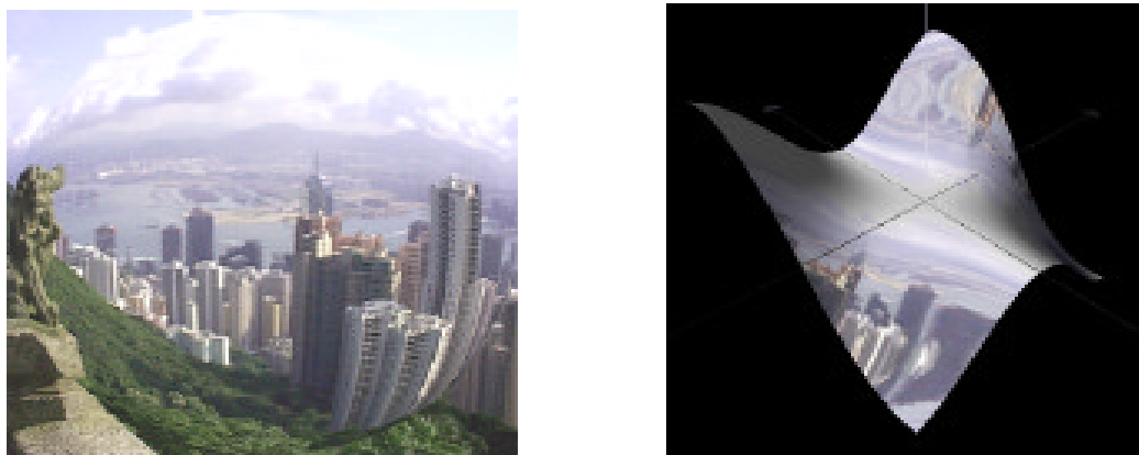
Figure 12.6: the original texture for an environment map (left) and the map on a surface (right)
